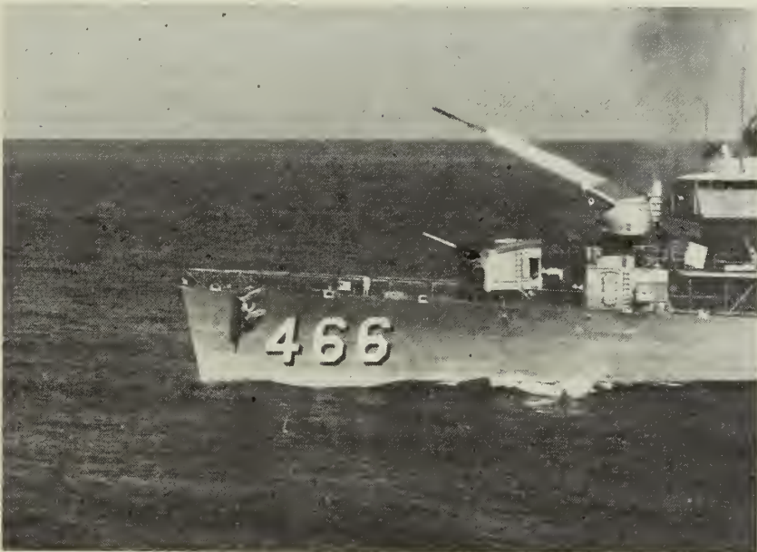
SCRATCH ONE SUB—Escort destroyer USS Waller (DDE 466) launches weapon Alfa, a long-range antisubmarine rocket, during ASW exercise in Atlantic.
